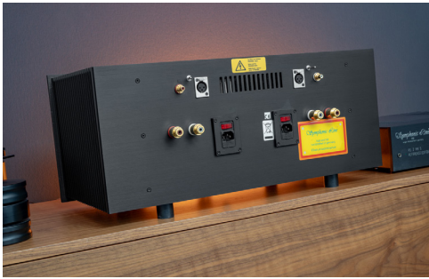
On the back, the double-mono design of the Kraft 300 Class A Anniversary Edition MK 3 becomes apparent: The case houses two completely independent mono blocks which, consistent with the model's design, each have their own power supply and even their own mains connection. The yellow Symphonic Line sticky pad is part of the sound optimization by Rolf Gemein.
